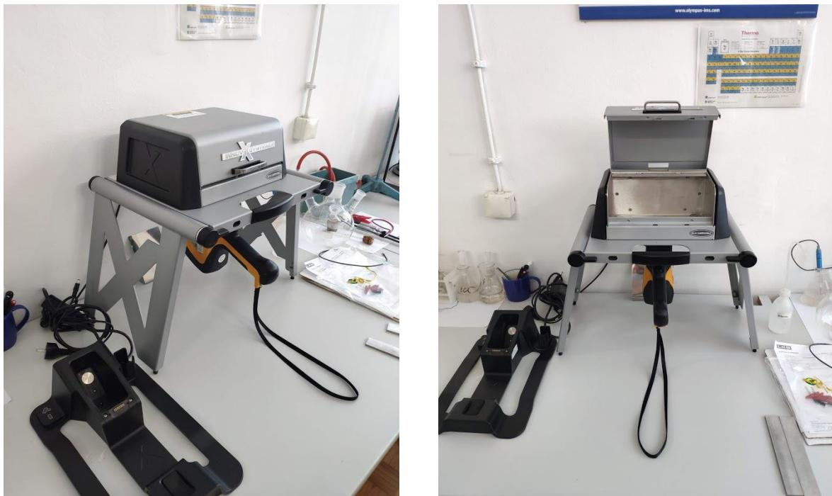
Slika 5.3 XRF analizator Innov - X Systems
