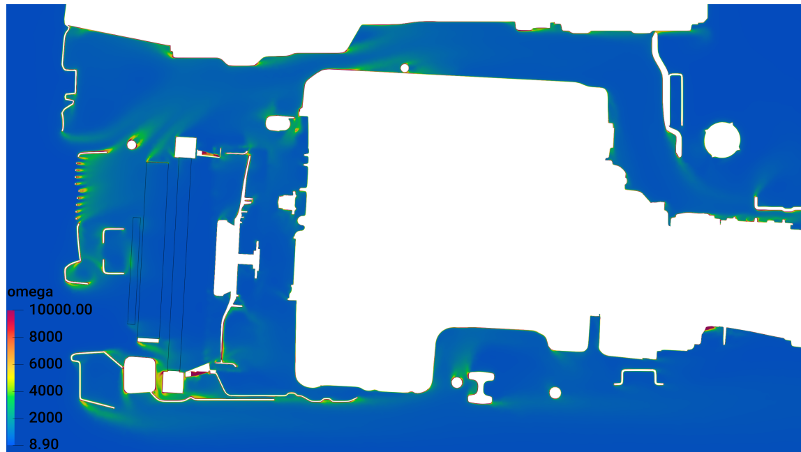
Figure 5.2.5: Ford Otosan truck cold flow, cross section: specific turb. dissipation rate.
