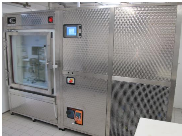
Figure 8. “HKS 700” climatic test chamber
