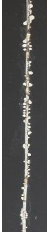
Figure 63. Delamination pattern around the scribe line on COB after 480 h of CH test
