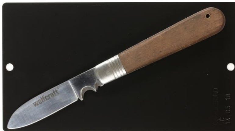
Figure 28. “Wolfcraft” knife used to scratch the specimen surface
