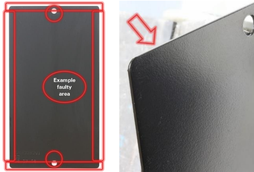
Figure 22. Example specimens with marked areas, which are excluded from the degree of rusting evaluation
