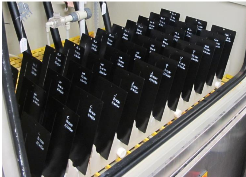
Figure 41. Placement of the specimens in the PV 12010 test chamber
