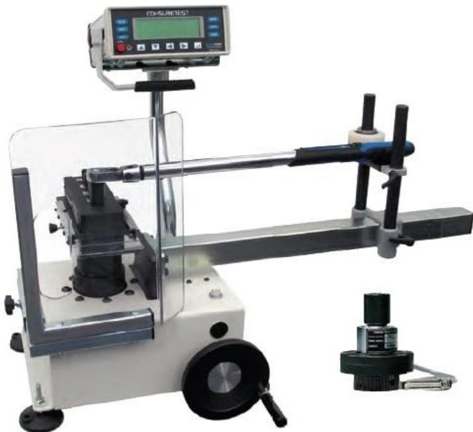
Slika 10. CDI Basic Suretest Torque Calibration System - 5000 -3 [2]
