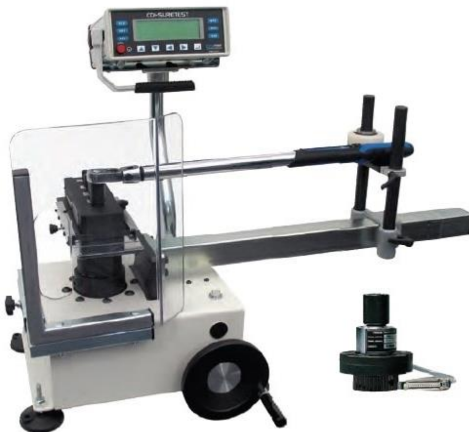
Slika 10. CDI Basic Suretest Torque Calibration System - 5000 -3 [2]
