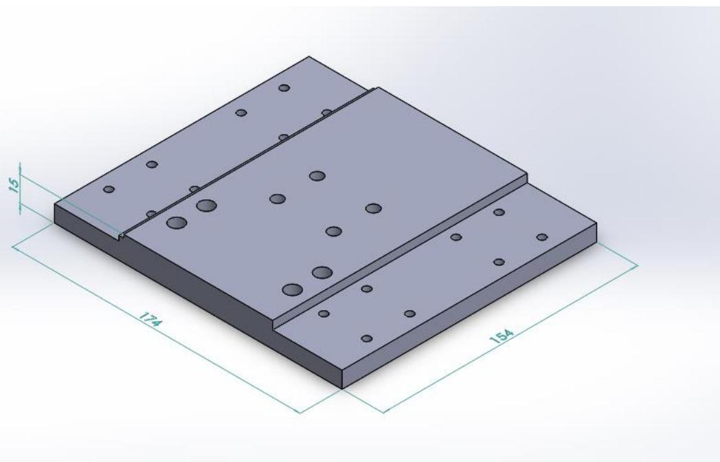
Slika 46. CAD model klizne platforme
