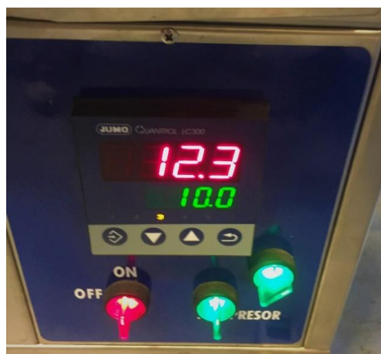
Slika 4. JUMO QUANCONTROL LC300 regulator temperature
