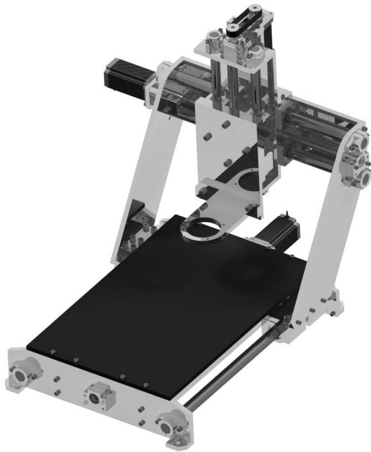
Slika 47. Render 3D modela CNC glodalice(1)
