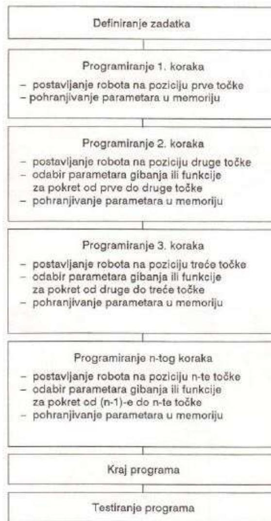
**Slika 4.4 Blok dijagram programiranja robota metodom *teach in* [17]**
