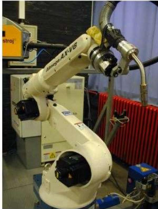
Slika 5.2 Robot OTC ALMEGA AX-V6 [20]
