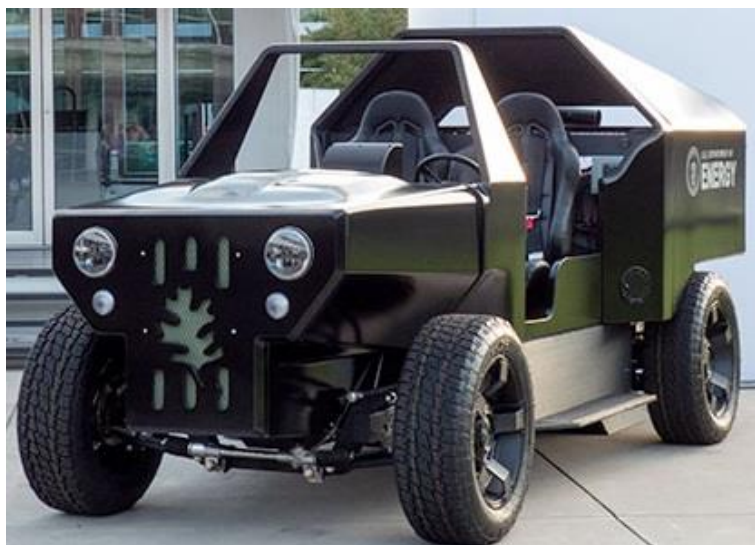
Slika 2.16. PUV (Printed Utility Vehicle) [33]
