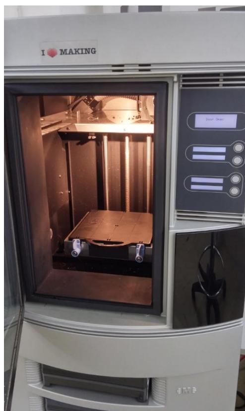
**Slika 27 FDM 3D printer Dimension Elite (IZIT)**
