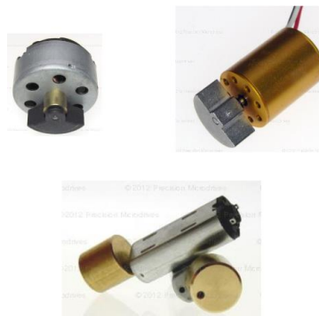
Figure 12.ERM actuators [Source: Precision Microdrives]
