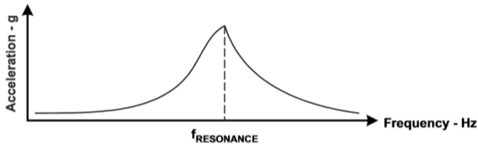
Figure 16. Typical LRA Response [30]
