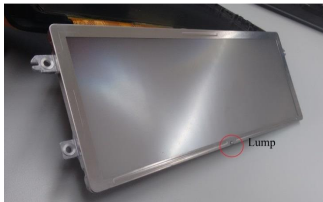
Separated backlight (used for the prototype)
