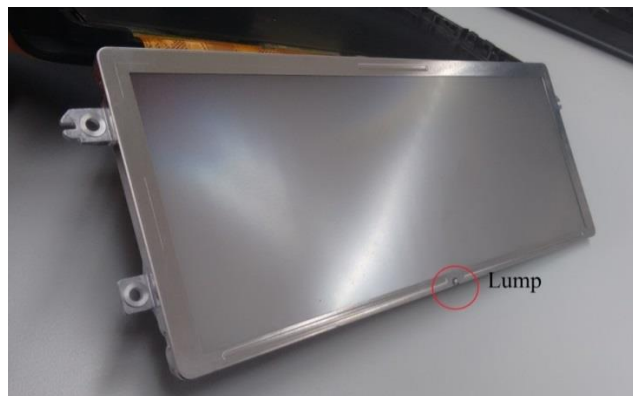
Separated backlight (used for the prototype)
