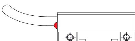
Red LED = poor signal strength - adjustment required
