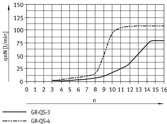
Standard flow rate  $q_n$  at 6 → 0 bar
