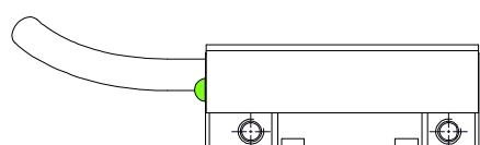
Green LED = good signal strength / set-up
