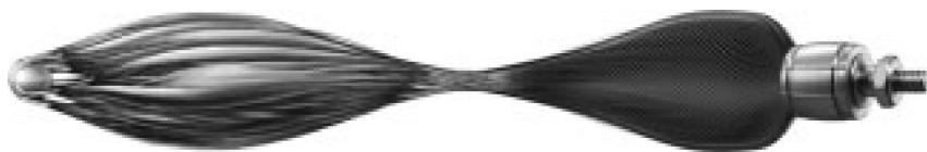
Fluidic Muscle is a tensile actuator which mimics the natural movement of a muscle. It consists of contractile tubing and appropriate connectors. The contractile tubing is made up of a rubber diaphragm with a non-crimped fibre made of aramid yarns on the inside. The diaphragm provides a hermetic seal enclosing the operating medium. The yarns serve as a reinforcement and trans-
