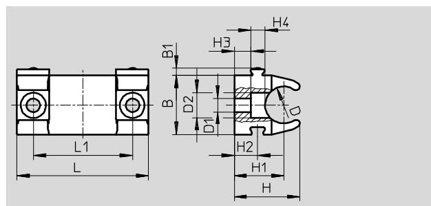
Linking of multiple retainers via dovetail slot
