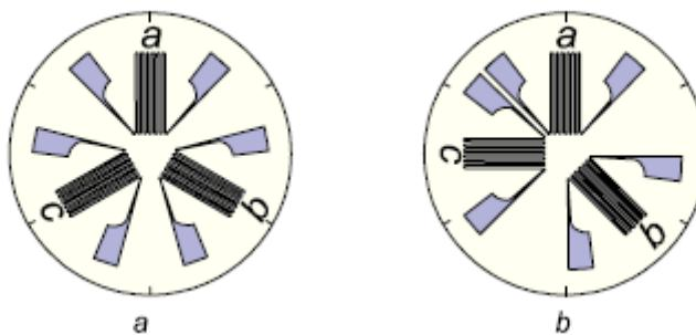
**Slika 4.6.** Mjerna rozeta: a) ( $0^\circ/60^\circ/120^\circ$ ) i b) ( $0^\circ/45^\circ/90^\circ$ ) [10].
