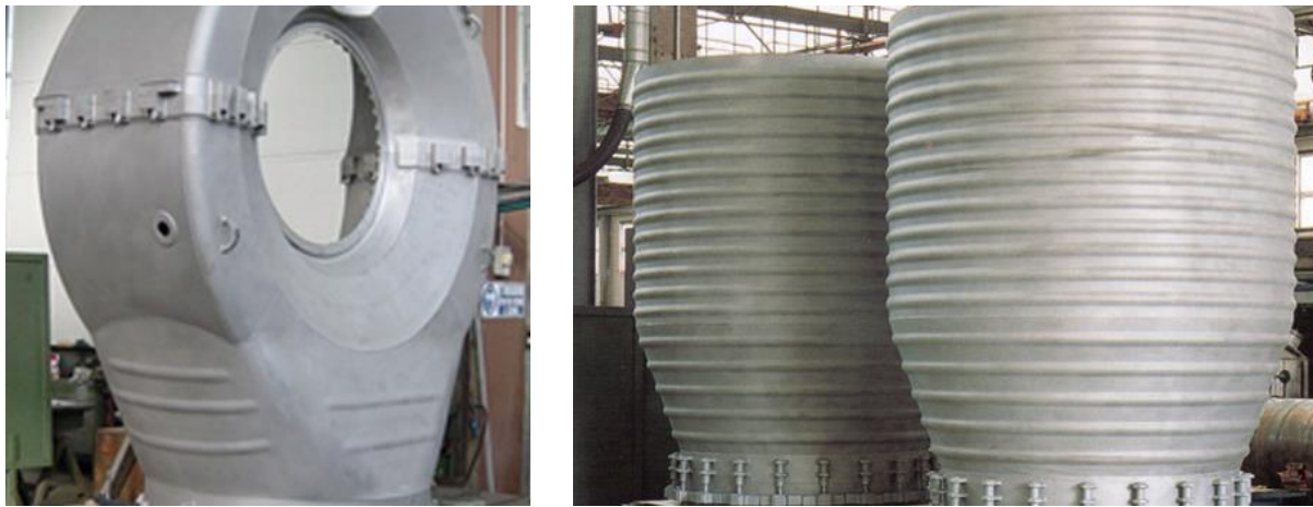
Figure 3. Hot gas casing and combustion inner liner
