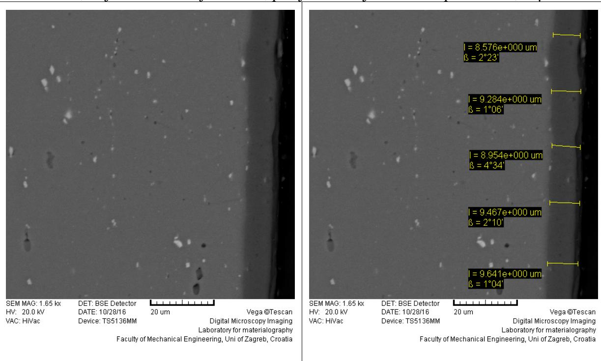
**Uzorak O2; vrijeme anodizacije: 30 min; prosječna debljina oksidne prevlake: 7,844 µm**
