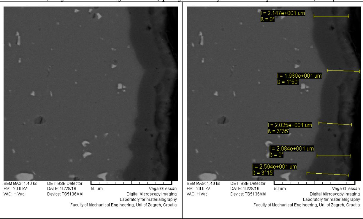
**Uzorak S3; vrijeme anodizacije: 20 min; prosječna debljina oksidne prevlake: 6,532 µm**
