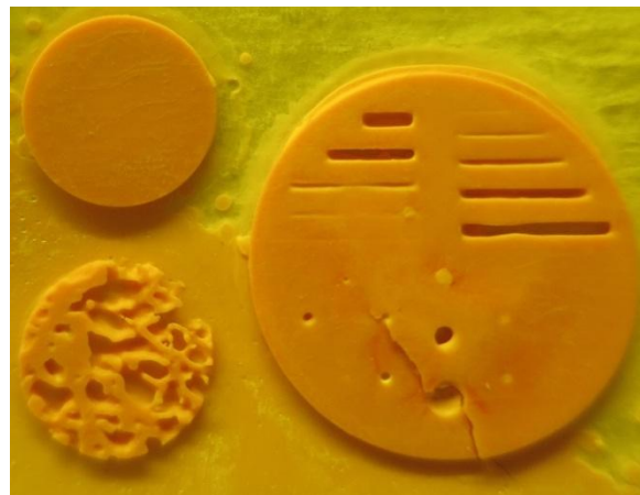
Figure 43. Printing quality with absorber content of 0,018 wt%
