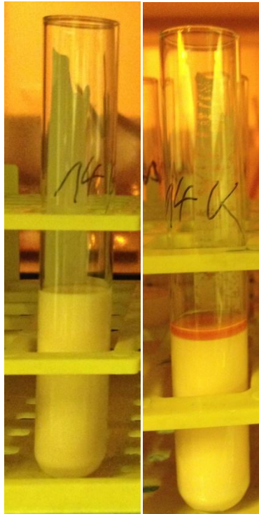
Figure 11. Room temperature stability of the original slurry
