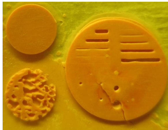
Figure 43. Printing quality with absorber content of 0,018 wt%
