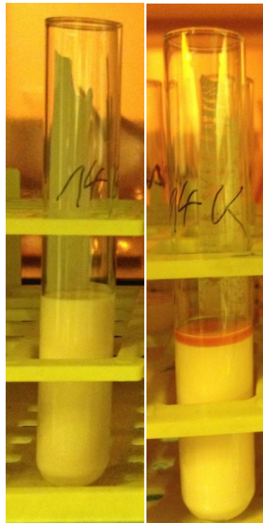
Figure 11. Room temperature stability of the original slurry
