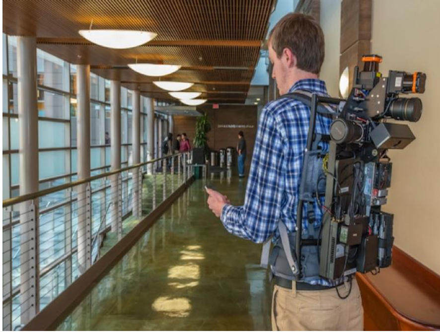
Figure 6 Rapid Building Energy Modeler (RAPMOD) (source:[17])
