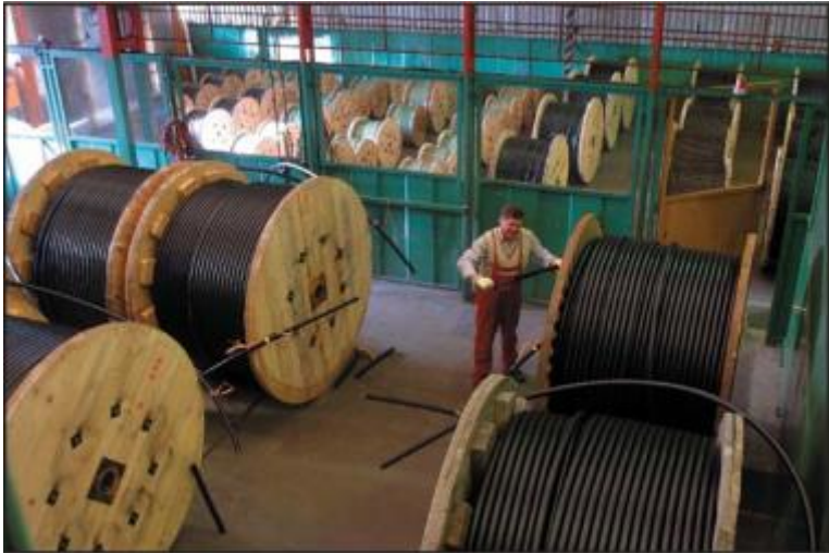
Figure 44. Wooden drums for cables
