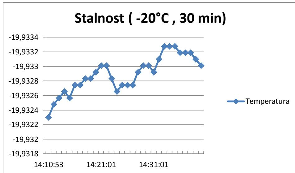
Slika 14: Stalnost temperature za  $-20^{\circ}\text{C}$  - kupka Kambič/etanol
