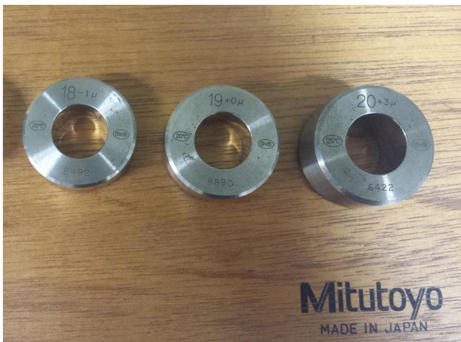
Slika 44. Mjerni kontrolni prsteni promjera  $\varnothing 18 \text{ mm}$ ,  $\varnothing 19 \text{ mm}$  i  $\varnothing 20 \text{ mm}$
