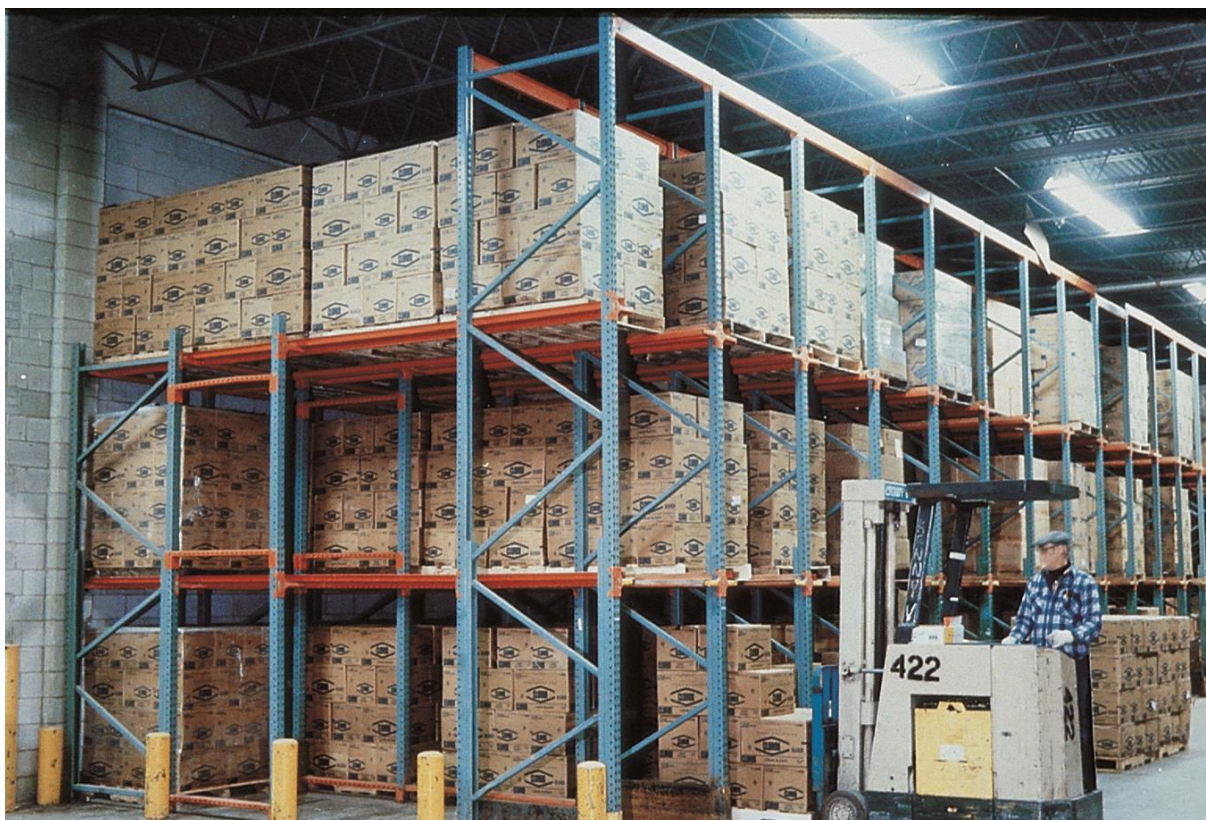
Slika 8. Prolazni regali (eng. Drive-In Rack, Drive-Through Rack ) [9]
