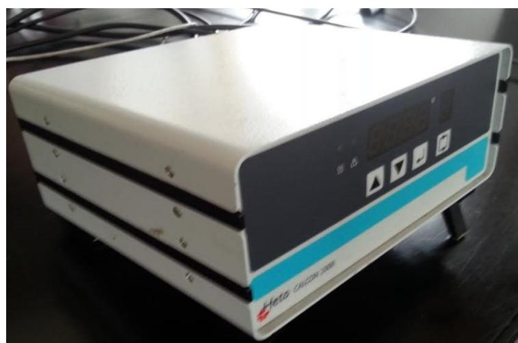
Slika 6. Calcon 2000, regulator temperature
