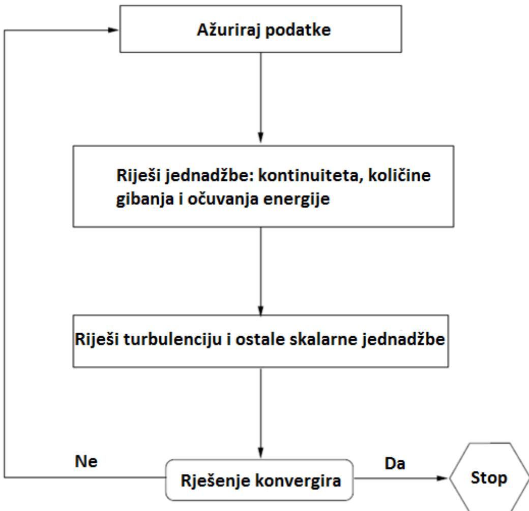
Slika 14. Logički dijagram - density based solver
