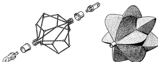
Slika 2.9. ROMAC (RObotic Muscle ACTuator) pneumatski mišić [6]
