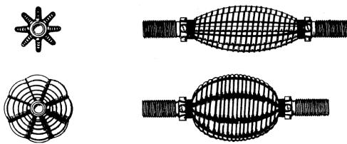
Slika 2.10. **Yarlottov pneumatski mišić** [6]
