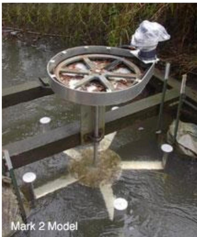
Slika 25. Alternative Hydro solutions Darrieusova turbina
