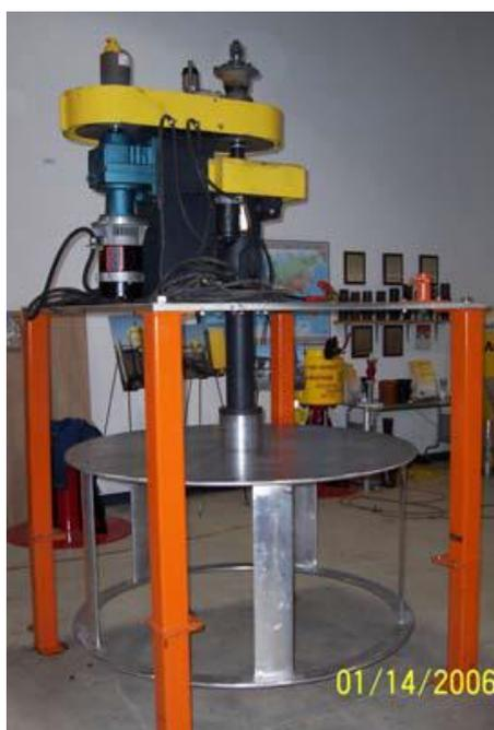
Slika 9. EnCurrent Squirrel cage Darrieusova turbina [4]
