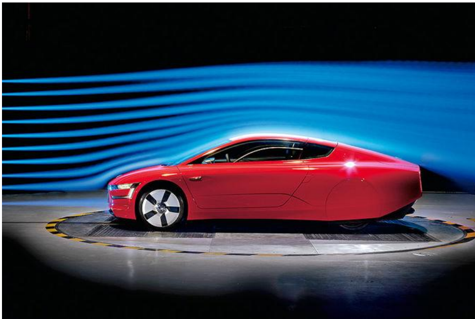
Figure 1.5 Low drag vehicle during wind tunnel test (VW XL 1, 2012) [14]
