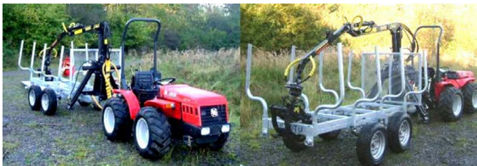
Slika 24. Prikolica Riko Fast Tow Forwarding trailer [16]
