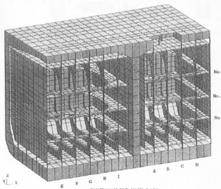
Finite Element Model, hull & tank
