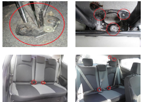
Figure 25: Improperly secured bench seat (top), improperly fitted third seatbelt on the rear bench seat of Renault Clio III (bottom left) and properly fitted third seatbelt on the rear bench seat of Renault Clio III (bottom right).
