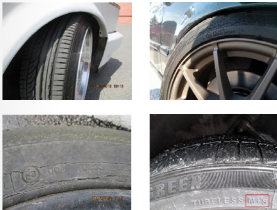
Figure 7: Tires that are too narrow with respect to the width of the wheel rim (top left), tires that get caught under the mudguards (top right), cracked and worn-out tires (bottom left), excessively worn-out tires (bottom right).
