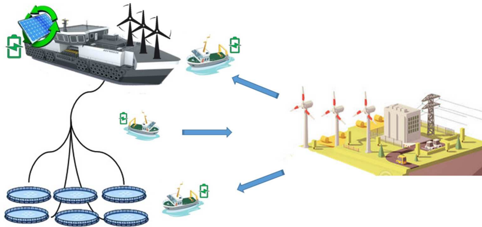
Figure 3. Model of an electrified mariculture system
