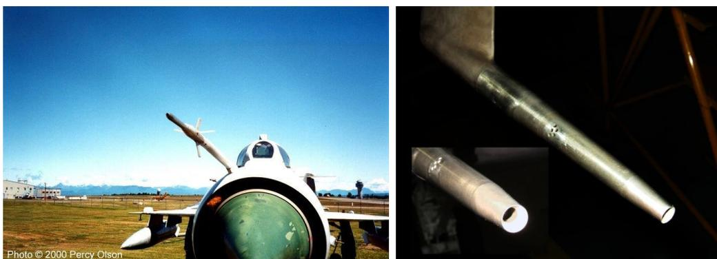
Slika 2.8 a) *Air data probe* zrakoplova Mig-21 [15]
