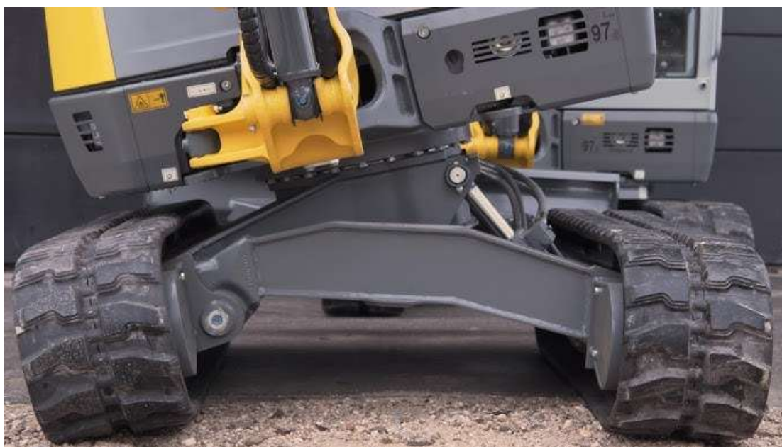
Slika 9. Wacker Neuson, Vertical digging system [16]
