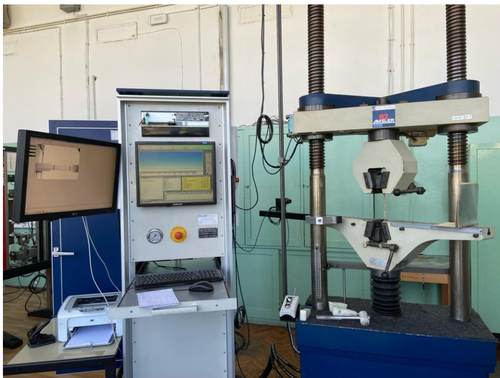
Slika 6. Amsler ADR – TS – 100THZ 100 kN
