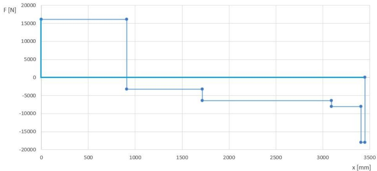
**Slika 49.** Dijagram raspodjele poprečnih sila
