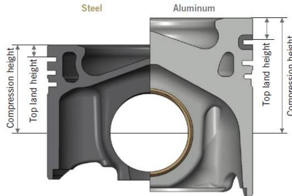
Figure 17. Geometrical comparison of steel and aluminum pistons [8].
