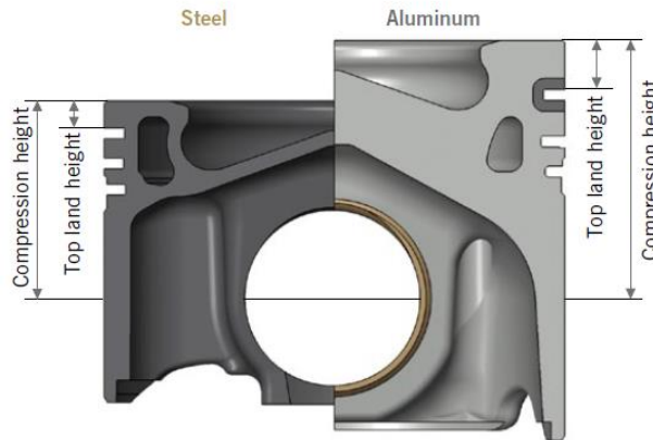
Figure 17. Geometrical comparison of steel and aluminum pistons [8].
