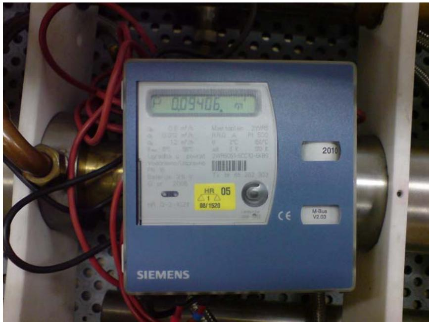
Slika 8.6 Kalorimetar SIEMENS 2WR5 u testnom modu
