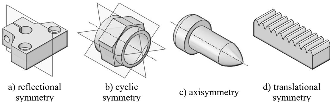
Figure 2. Mechanical parts with diverse types of symmetries
