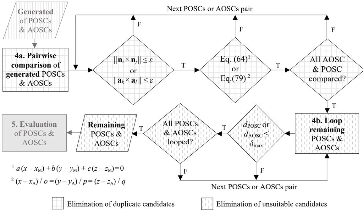
Figure 24. Flowchart of the candidate trimming step
