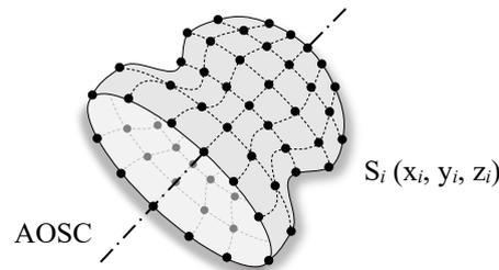
Figure 73. A uniformly sampled axisymmetric face
