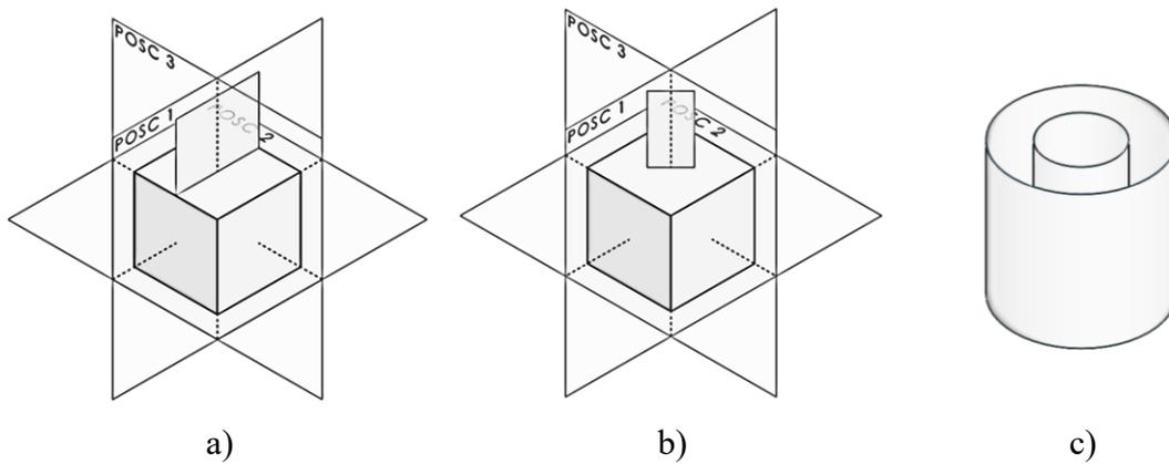
Figure 62. Examples of non-manifold 3D CAD models
