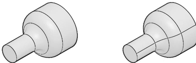
Figure 14. Example of unpartitioned (left) and partitioned periodical faces (right)
