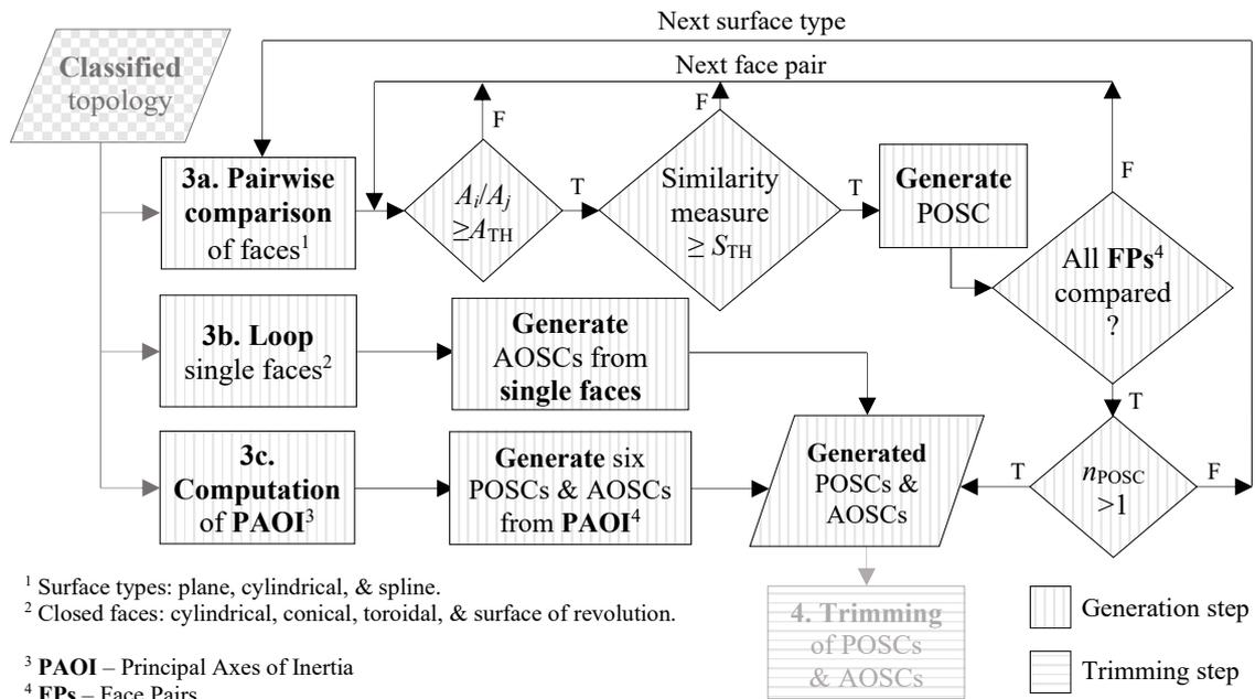
Figure 18. Flowchart of the candidate generation step
