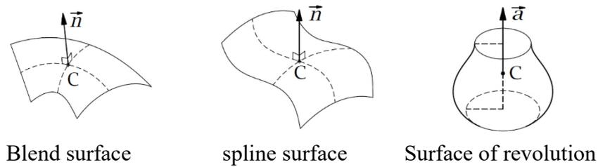
Figure 16. Examples of different types of numeric surfaces
