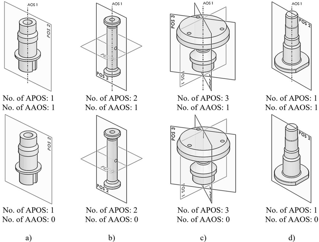
Figure 60. Symmetry detection results with (upper row) and without (lower row) the sub-step generation of candidates from single faces
