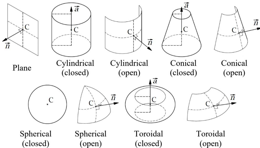
Figure 15. Examples of different types of analytical surfaces
