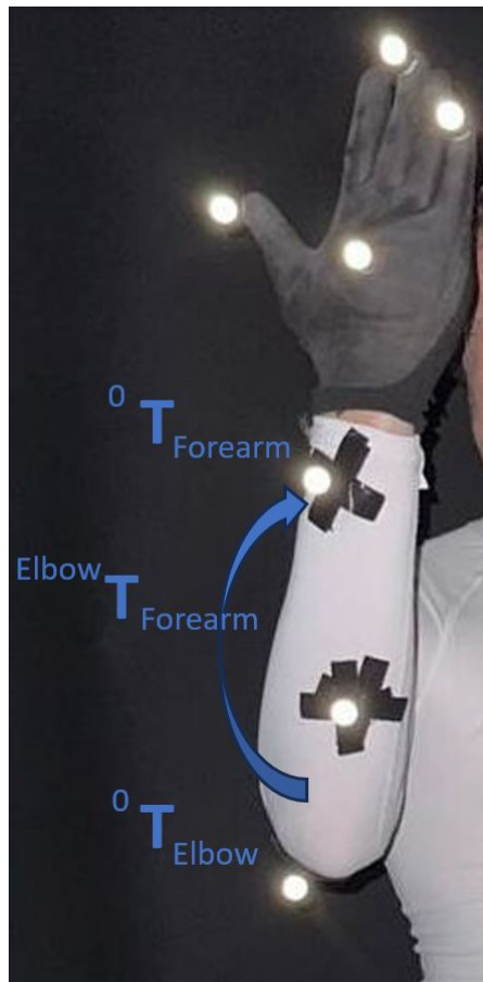
Figure 5.6: Example of calculating the transformation matrix that describes the relation between the marker on the elbow and forearm segment
