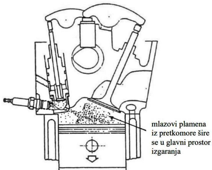
Slika 6. Jet Ignition motor, LAG, L. Gussak [4]
