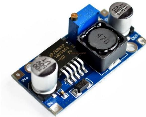
**Slika 15. DC-DC Buck konverter LM2596s [9]**
