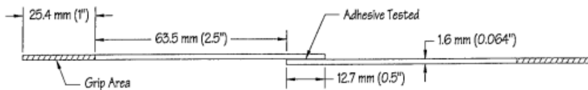
Figure 4. ASTM D1002 specimen [13]
