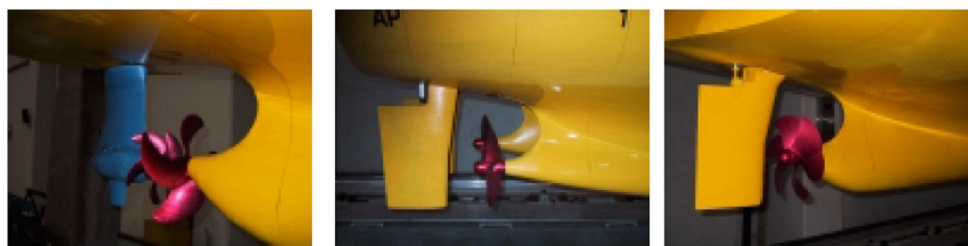
Figure 2. CRP Azipod® model.
