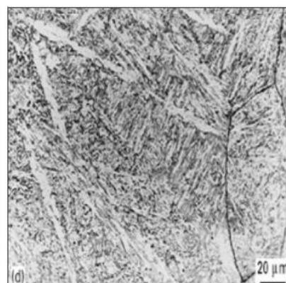
$T_A=1250\text{ }^{\circ}\text{C}$ , 580 HV
