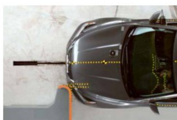
Driver-side small overlap frontal test configuration
