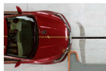
Passenger-side small overlap frontal test configuration
