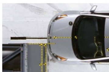
Moderate overlap frontal test configuration
