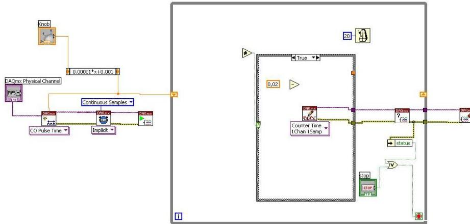
Slika 5.27. Shift register, Not Equal i Subtraction modul
