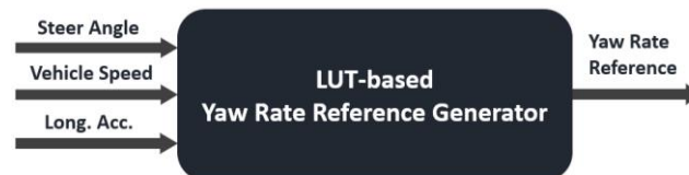
Figure 26. Proposed LUT-based yaw rate reference generator
