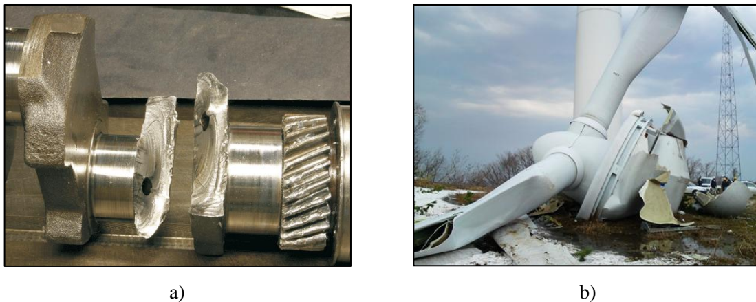
Figure 4. Fatigue failure of components: a) crankshaft [57] and b) wind turbine [58]
