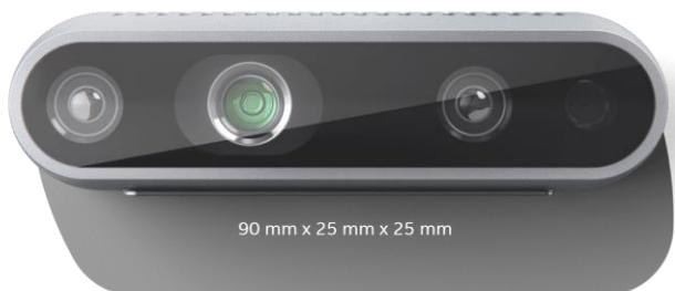
Slika 3.10 *Intel Realsense D435* [27]
