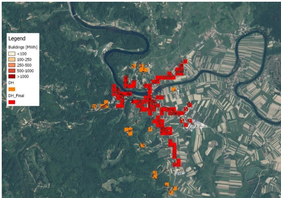
Figure 6 Parts of the city in which it is feasible to connect to a district heating system (orange) and final selection used in the further analyses (red)
