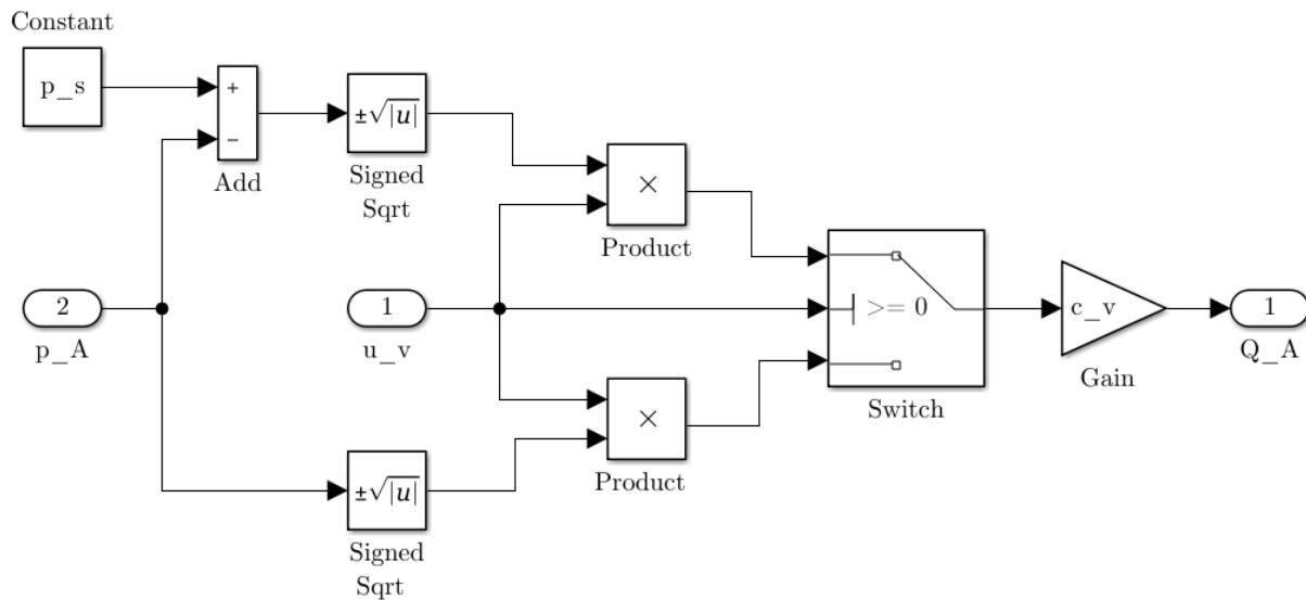
Slika B.10: Simulacijski model protoka  $Q_A$  kroz ventil
